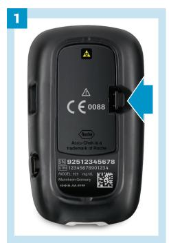
Open the battery door on the back of the meter by pushing the tab in the direction of the arrow and pulling the door up.
