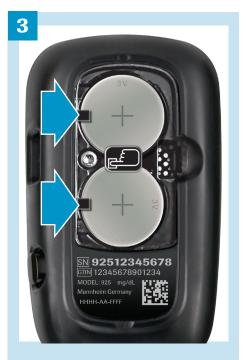
Slide the new batteries under the black tabs and button, with the (+) side facing up. Put the battery door back in place and snap it closed.
