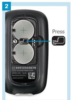
Release the old batteries by pressing the button. Remove the old batteries.
