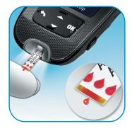
Touch the **yellow edge** of the test strip to the blood drop. Remove your finger from the test strip when "Analyzing" appears on the display.
